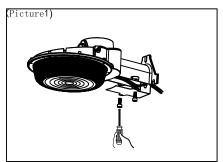
1. Use tools to remove two screws and covers from the luminaire. (as shown in the picture)
