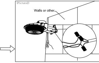
2. use tools to drill three holes on the wall. Then mount the canopy and luminaire to the wall after that ,connect the power lead to branch circuit at last,seccured the covers to luminaireby screws Note:Alisted canopy(IFFX/7)Must be provided by client.
