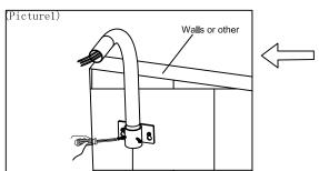
1. Use professional tools to drill two screw holes on the wall. Install the bracket on the wall and tighten the screws. Then install the mounting arm on the bracket and fix it with two screws. (as shown in the picture)
