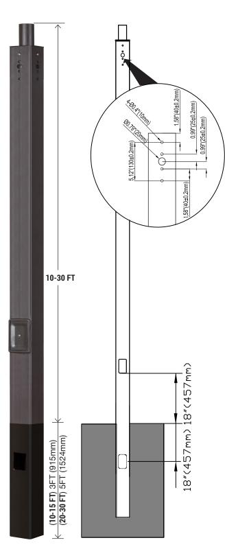
The WSD LED INC Series Direct Burial Straight Square Steel poles are built from high strength steel tube and are available side drilled for arm mounted area lighting luminaires or with tenon mounts for flood and post top luminaires. Typical area lighting applications include retail centers, industrial parks, schools and universities, public transit and airports, office buildings and medical facilities. Mounting heights of 10 to 30 feet can be used based on selected luminaire application.
