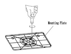
2. Securely attach mounting plate to J-box (not provided).
