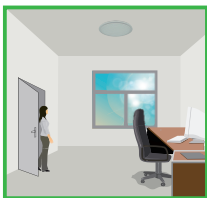
With sufficient natural light, the light does not switch on when presence detected.
