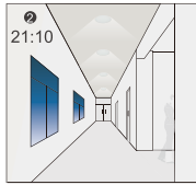
The light dims to stand-by level after the hold-time.
