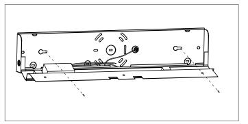
5.Rettach the driver cover assembly to the luminaire housing, and then pressing the cover back until it is retained by the slots.
