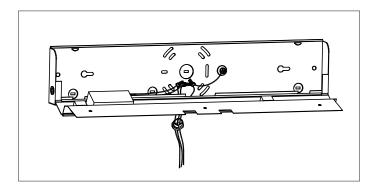
6.Reattach the lens onto the luminaire housing.
