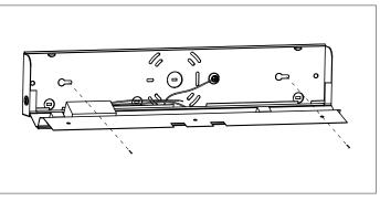
5.Rettach the driver cover assembly to the luminaire housing, and then pressing the cover back until it is retained by the slots.
