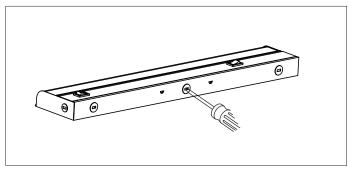
3.Position the luminaire housing in the desired location, and then mark and drill mouting holes at the narrow ends of the keyhole slots.Screw in mounting screws leaving space for channel body.Slide channel over mounting screws. Lift and shift channel into position and tighten screws.
