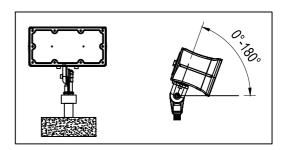
B 1.Drill 8mm hole on the wall or ground, please make sure the position of the crew hole match with the following dawing
