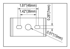
2.fixed the bracket on the crew hole,and adjust the angle of light according to your application, fasten the crew in the middle of adjustable arm,then Connect AC power wire.make sure all connection is fine,
