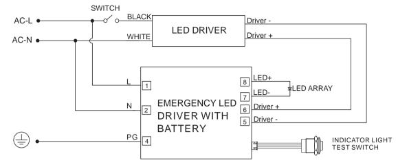
1.DO NOT MATE CONNECTOR UNTIL INSTALLATION IS COMPLETE AND AC POWER IS SUPPLIED. 2.TEST ACCESSORY LEADS-OBSERVE PROPER POLARITY WIRING.
