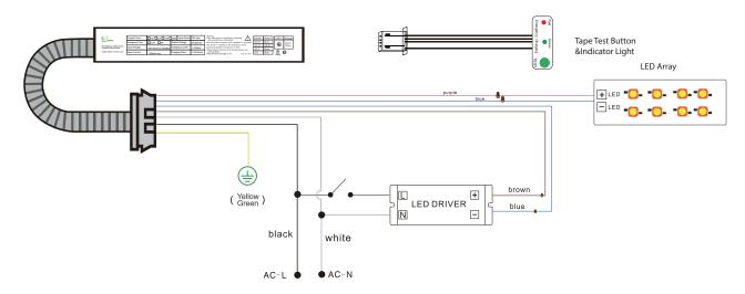
1. IN EMERGENCY MODE, DOUBLE-CLICK THE TEST SWITCH TO TURN OFF THE CURRENT EMERGENCY STATE.
