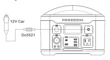
A. Plug the original car charger into the cigarette lighter socket of your 12V car, and then plug into the DC input port of the machine. B. The original car charger features 15A protector tube to protect your car.
