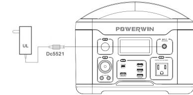
Plug the original adapter into the machine's DC input port and you will see the battery indicators on the screen blink.
