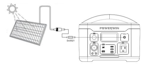
A.Place your solar panel where it will get as much strong direct sunlight as possible. B.Connect the output port of the solar panel with the input port of the product to start charging. You will know the product is being charged when the LCD display indicators blink. The product is fully charged when all battery indicators stop blinking and remain solid.
