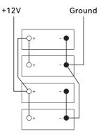
Parallel charging (Max 4S4P) can improve the consistency of the battery, and low-voltage charging is also safer, it should be noted that when charging in parallel, the cable should adopt the diagonal method toimprove the consistency of the current shunt. The so-called diaonal connection method is as follows.
