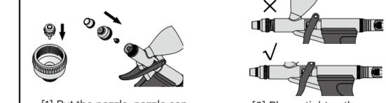
[1] Put the nozzle, nozzle cap and air cap back.
