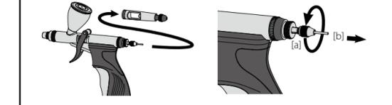
[1] Remove the handle. [2] Loosen the needle chucking nut[a], pull out the needle[b].
