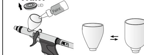
Put a few drops of paint in cup, dilute paints to look like milk if needed before pour into cup. This airbrush can be installed with different capacity cups to meet various spraying needs.
