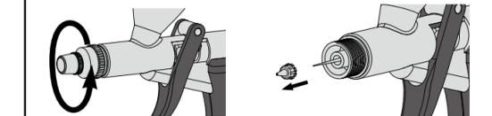
[3] Remove the air cap and nozzle cap. [4] Remove the nozzle.
