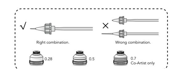
The package includes multiple sets of needles and nozzles of different sizes. Incorrect matching may result in either excessive needle exposure or inadequate exposure. Please ensure to store them separately.
