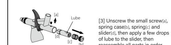
[3] Unscrew the small screw[a], spring case[b], and slider[c], then apply a few drops of lube to the slider, then reassemble all parts in order.
