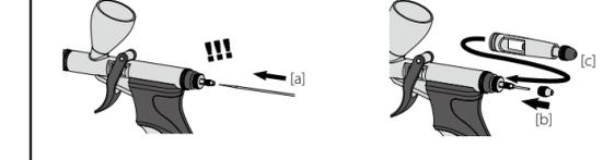
[3] Reinstall the needle[a], needle chucking nut[b] and handle[c]. Please avoid hitting the needle's front end.
