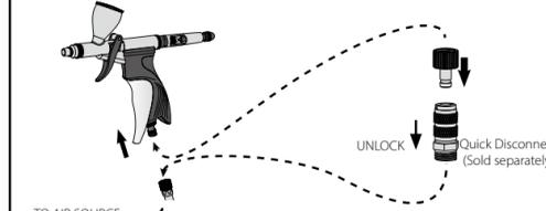
Begin by attaching the end of an airbrush hose (1/8" BSP) to your airbrush. Attach the male part to airbrush and the female part to air source, pull downside to unlock.
