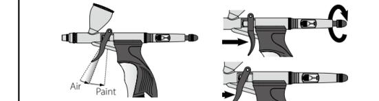
Turn your air compressor on. Pull back the trigger to release air flow, continue pulling to release paint flow. The preset fluid control knob (if equipped) can control the retracement of main lever.
