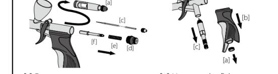
[1] Remove part[a] ~part[e]. [2] Unscrew the fixing nut[a] plastic handle[b], and value[c].
