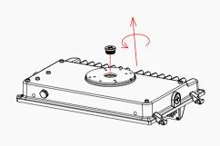
6.According to the embedded terminal box, punch the correspongding mounting hole on the light 's mount.
