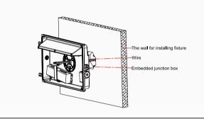
8. Usescrew to lock the lamp base on the embedded junction box, And ensure the balance of the horizontal column.
