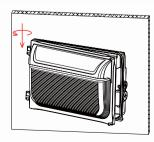
12.Lock the upper cover screws into the bottom shell with a cross screwdriver.
