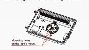
7.Put the input line in the embeddedbox passes through the waterproof pad and then passed through the lamp base.
