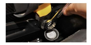
2. Use an E12 socket with a 3/8 inch wrench and extension bar to remove the four seat bolts on both sides of the seat tracks. You can slide the seat forward and backward for better access to the bolts.
