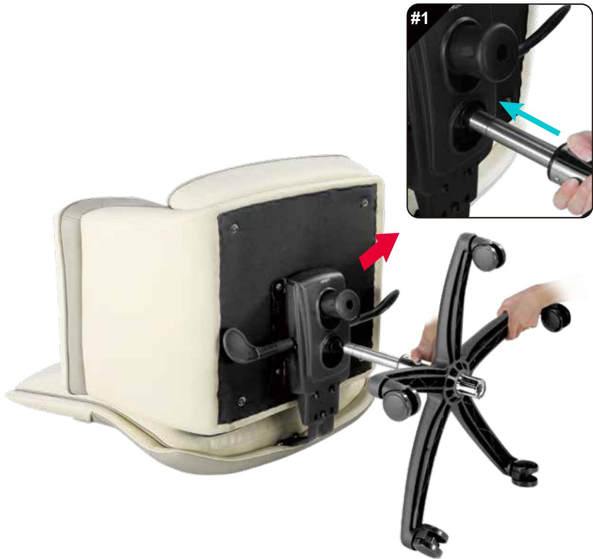
Insert the gas cylinder into the socket of the tilt mechanism.
