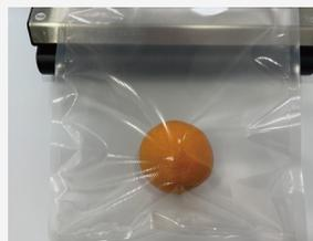
2. Open the lid and place the opening end of the bag into the Vacuum Chamber.
