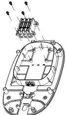
4.1.2 Find the wall stud nearest to the power supply wiring, place the wall-dock back panel to the wall stud and mark 4 mounting holes (M4), then remove the back panel.
