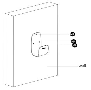
4.2.2 Drill 3 holes and insert 3 wall anchors into the mounting holes. Place the holster wall dock, then screw and tighten 3 Type C (M4 x 30 mm) screws into the mounting holes.
