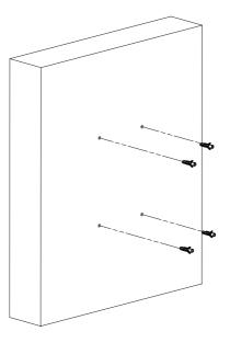
4.1.4 Place the back panel, then screw and tighten 4 Type C (M4 x 30 mm) screws into the mounting holes.
