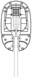
4.1.6 Align the charging station with the wall-dock back panel, gently insert and assemble.
