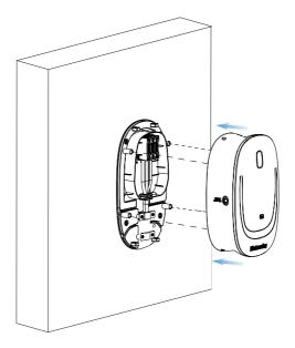
4.1.7 Screw and tighten the charging station into the wall-dock back panel using 4 Type A (M4 x 12 mm) screws.
