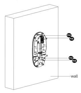
4.1.3 Drill 4 holes (M4) and insert 4 wall anchors into the mounting holes.
