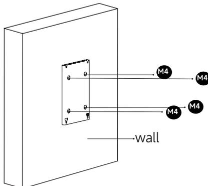
5.1.2 Drill 4 holes and insert wall anchors into the mounting holes. Attach the wall dock to the mounting location by screwing 4 Type B Screws (M4 x 30 mm) into the mounting holes then tighten them.
