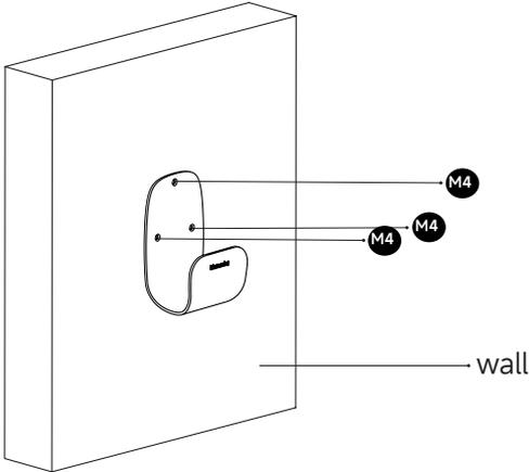
5.2.2 Drill 3 holes and insert 3 wall anchors into the mounting holes. Place the holster wall dock, then screw and tighten 3 Type B Screws (M4 x 30mm) into the mounting holes.
