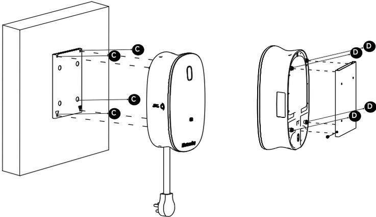
5.1.4 Screw the Type A Screw (M4 x 12 mm) into the hole at the side of the charger.
