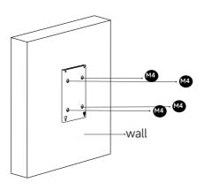
5.1.2 Drill 4 holes and insert wall anchors into the mounting holes. Attach the wall dock to the mounting location by screwing 4 Type B Screws (M4 x 30 mm) into the mounting holes then tighten them.
