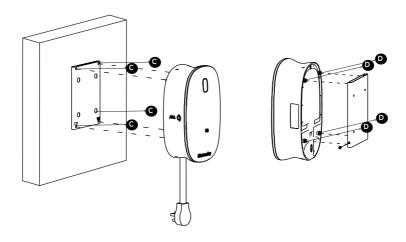
5.1.4 Screw the Type A Screw (M4 x 12 mm) into the hole at the side of the charger and tighten the screw to secure the charger.
