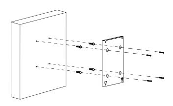
5.1.3 Attach the charger to the wall dock by inserting the mounting screws (D) on the back of the charger into the wall dock mounting holes (C). Slide the charger downwards.
