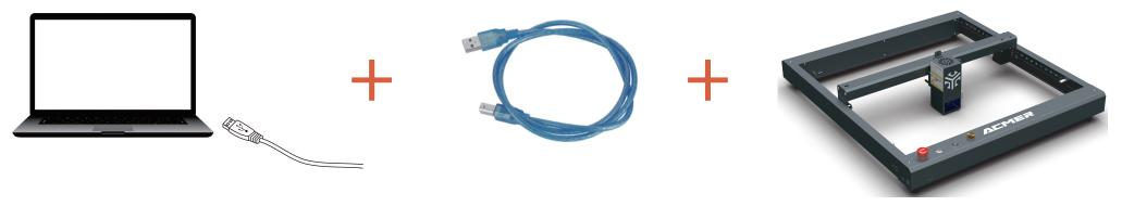
2. Open LaserGRBL software and select the correct port number and baud rate: software-115200
