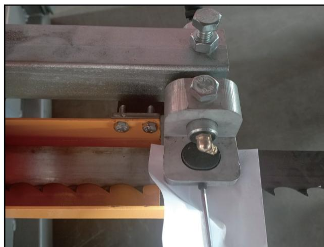
Adjusting the gap above the saw blade.
