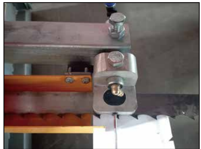
Adjust the gap below the saw blade.
