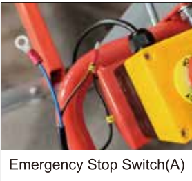
Step. 3: Find the Emergency Stop Switch(A) and the Micro switch (B)
