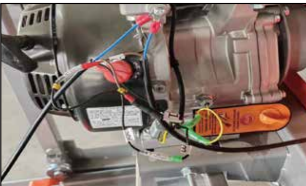
Step.5: Connect the A1 and 1 (Female) Connect the B3 and 3 (Male)
