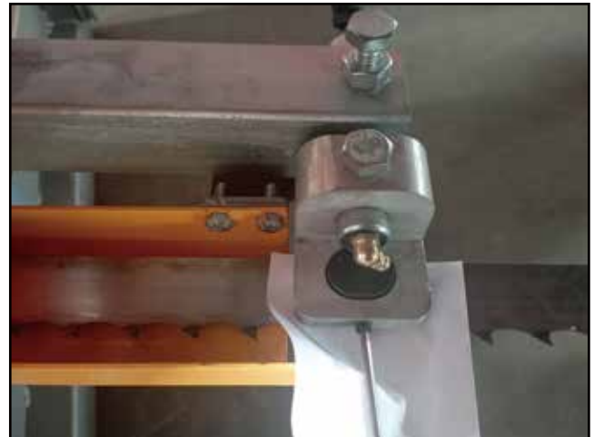
Adjusting the gap above the saw blade.
