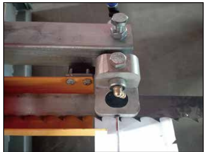
Adjust the gap below the saw blade.
