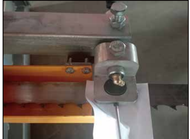
Adjusting the gap above the saw blade.
