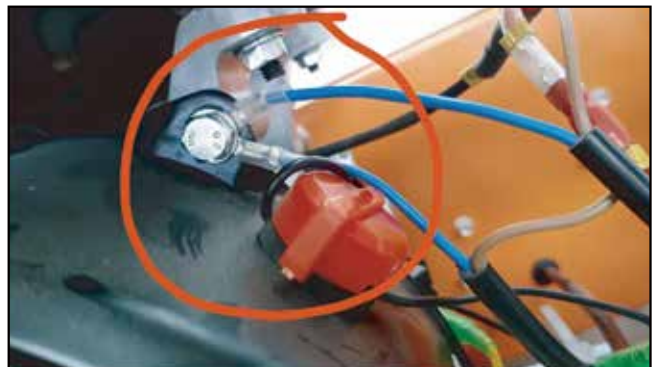
Step.6: Connect chassis
