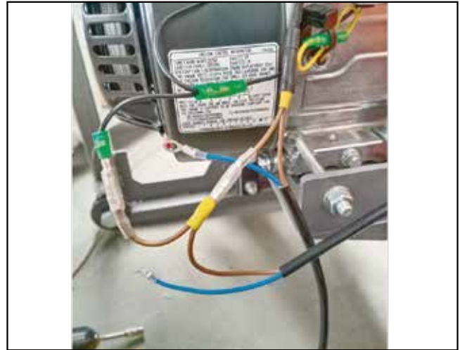
Step. 2: Disconnect BLACK(1and3) wire
