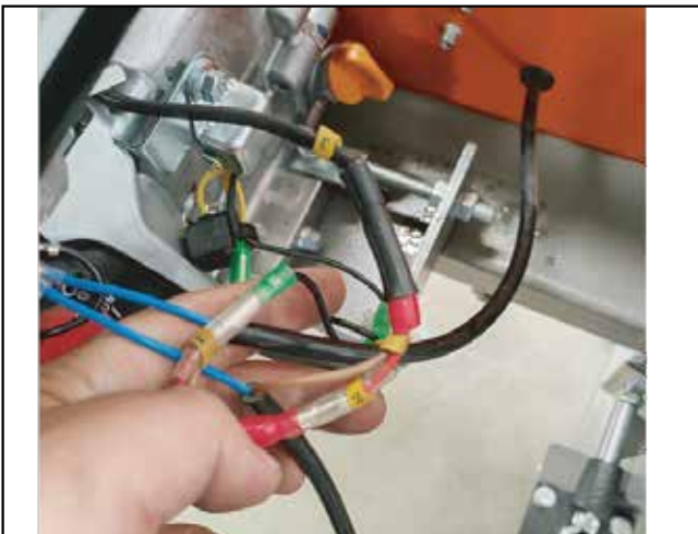
Step.5: Connect the A1 and 1 (Female) Connect the B3 and 3 (Male)
