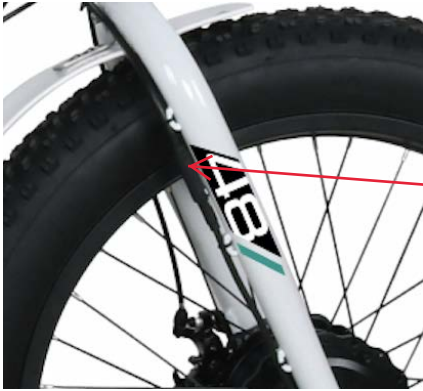
Quick Disconnect (front fork right side)
