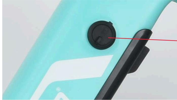
Slide open the protective hatch to access the charging port on the right side
