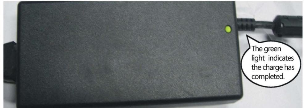
5. After charging completes, please pull out the charger power plug from the household AC and disconnect the plug from the battery
