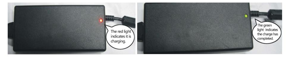
5. After charging completes, please pull out the charger power plug from the household AC and disconnect the plug from the battery
