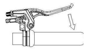
Pull to brake. Brake sensor will shut off motor power.
