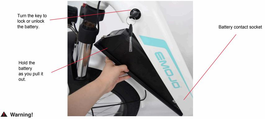
Note: While installing and removing, do not use extreme force to avoid damaging the battery pack and other components.
