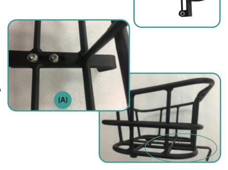
1-Fix the basket to the fork, use the long sockethead bolt and pass it thru the bracket tab (B) and into the fork, secure on the other side with a security nut.
