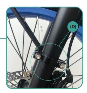
3-Attach the bracket rods to the bases already fixed on the fork. The rods ends should be attached on the inner part (E) Fully tighten all bolts now.
