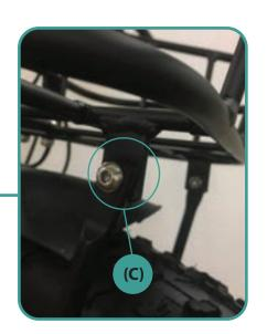
3-Attach the bracket fork bases (d) to the fork of your bike. This basket system now has an universal, fits models with bigger or smaller wheels. Adjust the height of the bracket bases accordingly. Make sure both sides are adjusted to the same height. Do not tighen yet.
