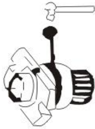
图六 榨条拆卸图 Squeeze the disassembly graph
