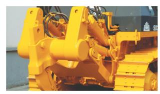
■ Large single-tooth ripper with the adjustable penetration angle is used to loosen the soil layers such as the clay and the frozen soil and to peel off the solid surface such as the gravels and the hardened salt mine. The work efficiency and the super penetration are guaranteed with the strength beam, the frame and the tempered tooth bar and tip.
