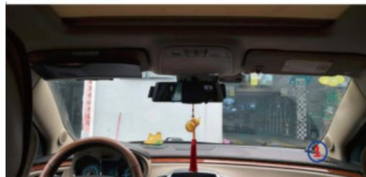
Position 1: Considering that the front windshield of a motor vehicle has a large enough view of the sky, it is usually recommended that the GPS module be placed in the central console. At the corners of the central console and the edge of the windshield, after adopting hidden wiring, they are fixed with double-sided tape.
