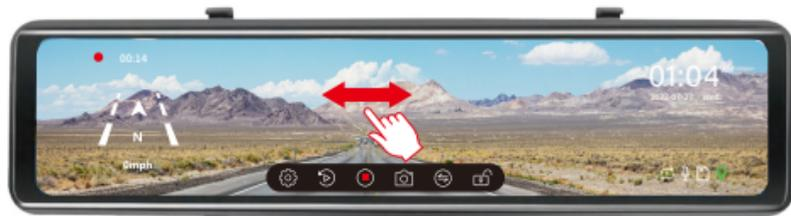
While recording, swipe the screen left or right to switch between front view, rear view, or split-screen view.
