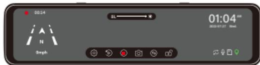
2) Once the GPS is installed, the GPS icon on the home screen will show. After the GPS signal has been received, it will show direction and speed.
