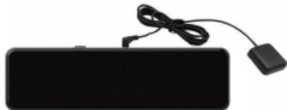
1) Install the GPS Antenna onto the camera, the GPS Antenna will start to search for a GPS signal.
