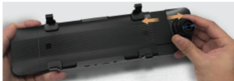
Step 2: Pull out the front lens of the T700 dash cam to match the rearview mirror of the vehicle.
