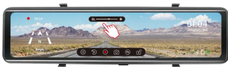
Touch the touchscreen to display the brightness scrollbar at the upper center, then slide right or left to adjust the brightness.
