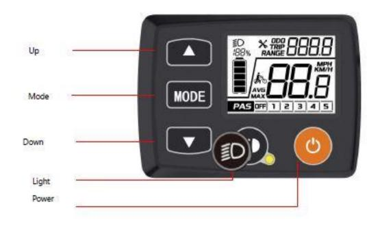
**Display Function** – Your Totem Osprey is equipped with a Vinka DR25 LCD Smart Display.
