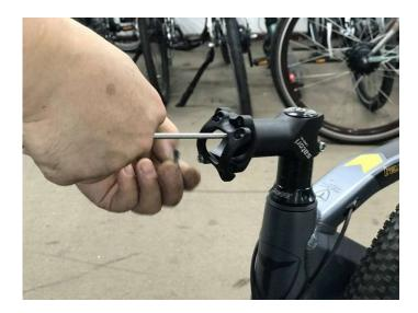
3. Mount and align the handlebars evenly both vertically and horizontally, then tighten the four screws.
