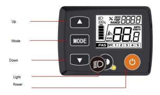
When the display is powered off you will see a blank screen. Using the orange power button, you can turn on the display.
