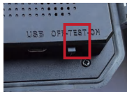
③ Switch to TEST
