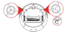
Please install the right brush into the right bottom mounting port of the machine, the left brush into the left botom mounting port of the machine, andensure that the two side brushes are in place.
