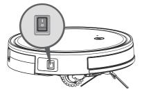
4. Long press "()" for 3 seconds, and then" ? "flashes, input the wi-fi account and password.(only support 2.4Ghz wifi,5Ghz can not be connected.) A few seconds later ,the product will be connected to your phone.
