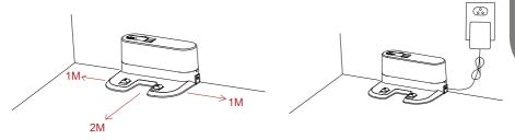
Turn on the side power switch, "I" is the turn, "O" is the turn off. After the finishes working, it is recommended not to shut down; keep the robot in a state of charge so that it can perform its next job better.
