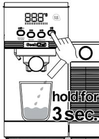
4. This clean cycle will run for 35 seconds and then stop automatically. Or press the Latte button again to stop process manually.
