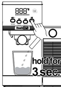
5. Press and hold the Cappuccino button for 3 seconds. The machine will start to make steam from the milk dispensing tube. This process will run for 2 minutes and then stop automatically. Or press the Cappuccino button again to stop process manually.
