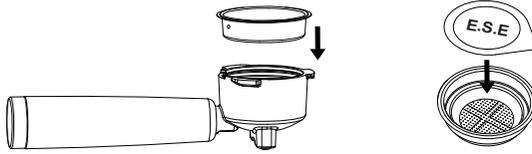
FOR A DOUBLE SHOT OR TWO SINGLE SHOTS – use the filter for a double shot of espresso. By placing two small cups underneath the filter holder, you may prepare two single shots of espresso at once.
