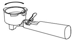
6. Insert the Filter Holder without coffee grounds into the Brew unit with a 45° movement to the left and turn it to the right to lock it in place. The filter holder handle must be perpendicular to the machine or slightly tilted towards the right.
