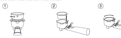
6. Insert the Filter Holder without coffee grounds into the Brew unit with a 45°movement to the left and turn it to the right to lock it in place. The filter holder handle must be perpendicular to the machine or slightly tilted towards the right.
