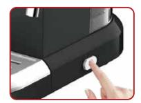
Plug in the power cord, 05 press ON/OFF button, all indicators will flash the machine is preheating.
