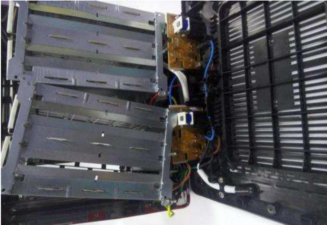
**Photo 34 - Internal view of Toaster, models WT-8200, WT-8200A, WT-8220, WT-8250, WT-8250A, WT-8250C, WT-8250B with grounding construction**
