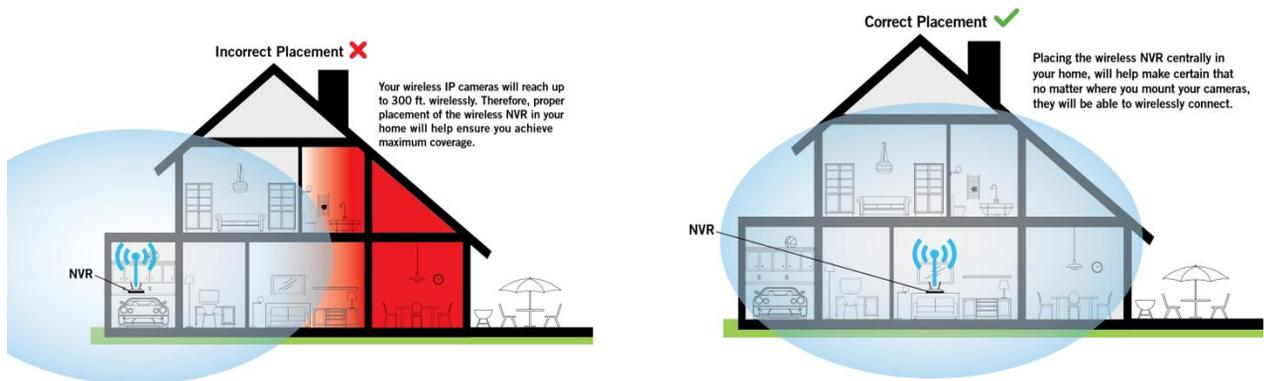
If there has to be obstacles between the NVR and camera, adjust the height of camera or NVR to avoid floor. Floors are normally heavier than walls.
