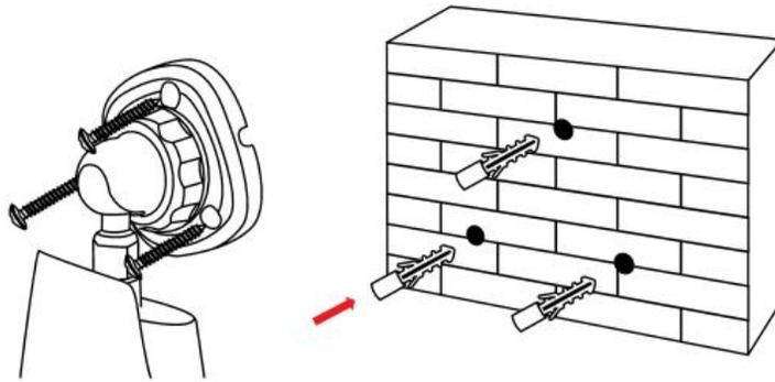
6. Once the base is screwed in place, make sure that the camera is securely mounted by placing gentle pressure on the mount.
