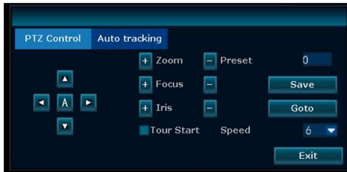
1. **Arrow Keys:** Allows you to move the camera up and down, left and right.
