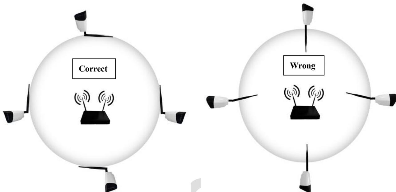
The NVR's antennas radiate signals to all around. The signal pick-up is best while antennas are on same height and parallel. If the cameras cannot be at same height with NVR, please keep their antennas parallel.
