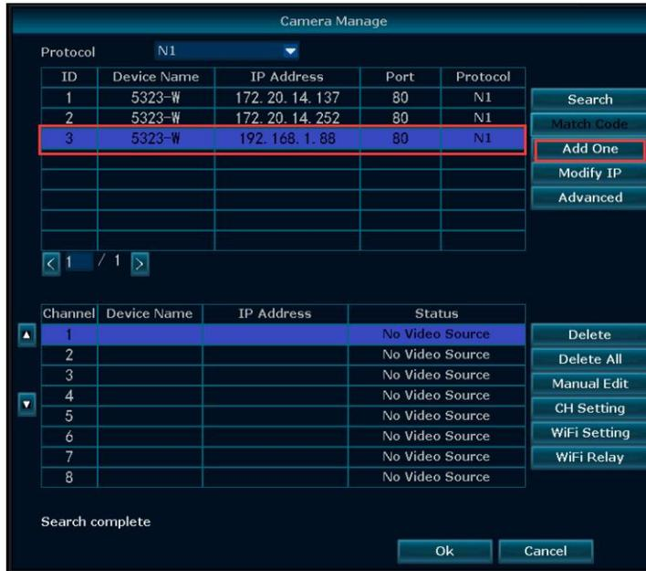
The camera's IP remains to be 192.168...now, your camera is streaming and working through the Ethernet cable. You can go ahead to mount the camera.
