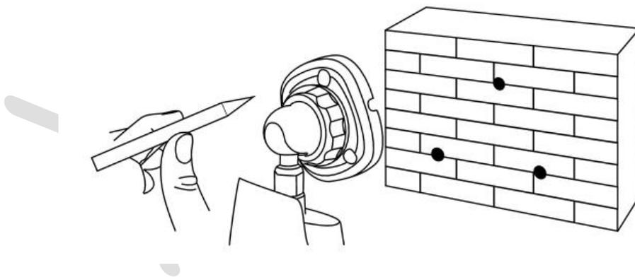
3. Using a drill bit slightly smaller than the included screw anchors, drill into the mounting surface using the guide marks you placed in the previous step.
