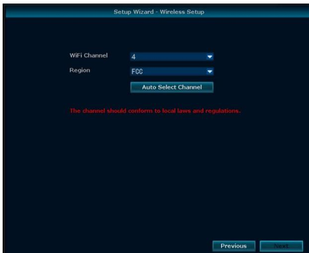
Wireless Setup will allow you to select a least-interfered WiFi channel for the NVR, ensures its performance not affected by other WiFi devices. Click "Auto Select Channel", the NVR will automatically select a WiFi channel with least WiFi interference.
