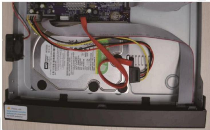
4. Holding the hard drive and NVR, gently turn it over and line up the holes on the hard drive with the holes on the NVR. Using a screwdriver, screw the provided screws into the holes. Assemble the cover.
