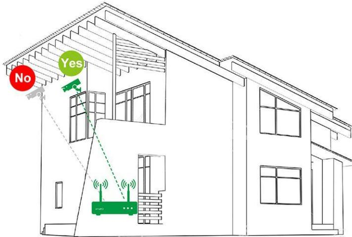
Metal walls (including metal garage gate) absorb wifi signal. Use extra extendable wifi antenna to bring camera's antenna inside the wall. This also works for heavy concrete wall.
