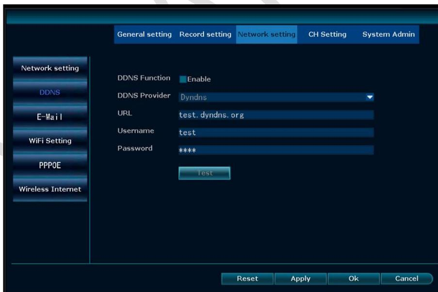
1. **DDNS Function:** Enable or disable the usage of the DDNS service on the NVR.
