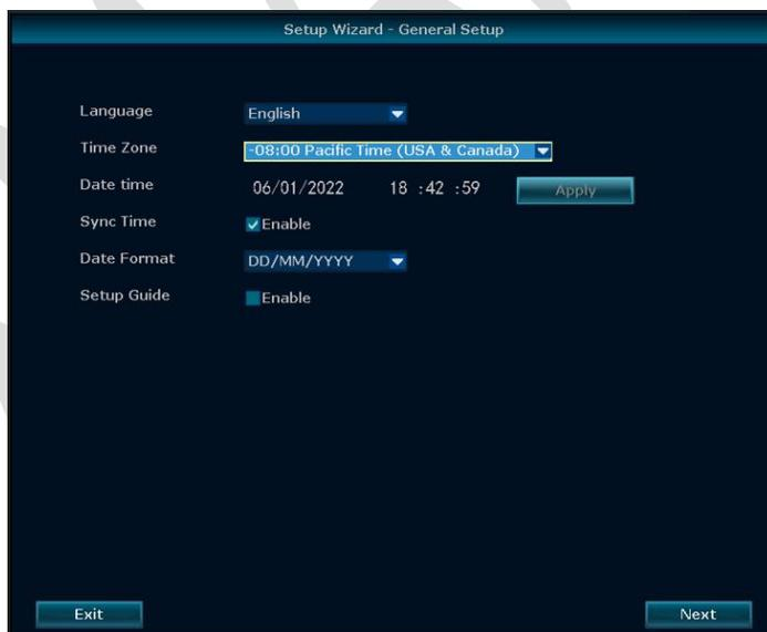
General Setup will allow you to set up NVR’s language, time zone, and date format. You may choose to use Network Time Protocol (NTP) to auto-configure the current date and time. To use NTP, check the Enable box next to **Sync Time**, then click **Apply**.
