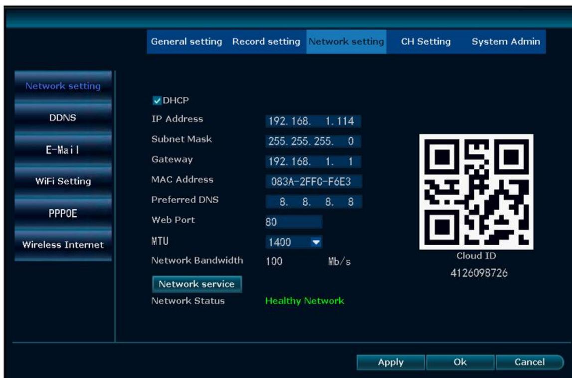
1. **DHCP:** Network configuration mode that gathers the network values automatically from DHCP server. If unchecked this value can be set manually.
