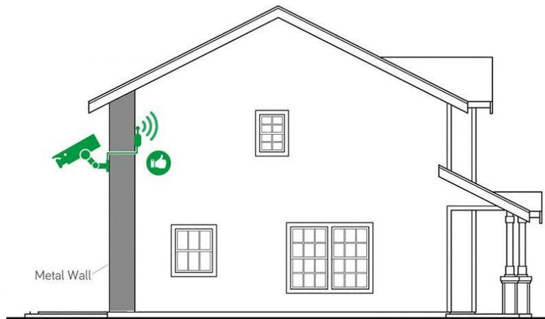
Try to keep camera and NVR's antennas parallel to get better signal pick-up.
