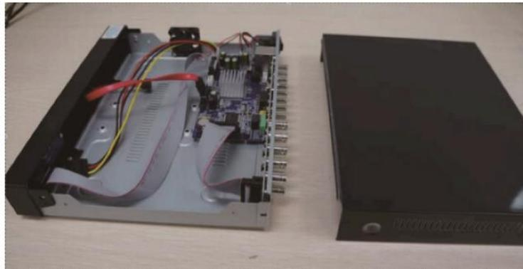
2. Connect the SATA power and data cables from NVR to the corresponding ports on your hard drive.
