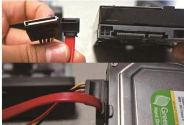
3. Place the hard drive into the NVR. Any cables should cross up over the HDD.
