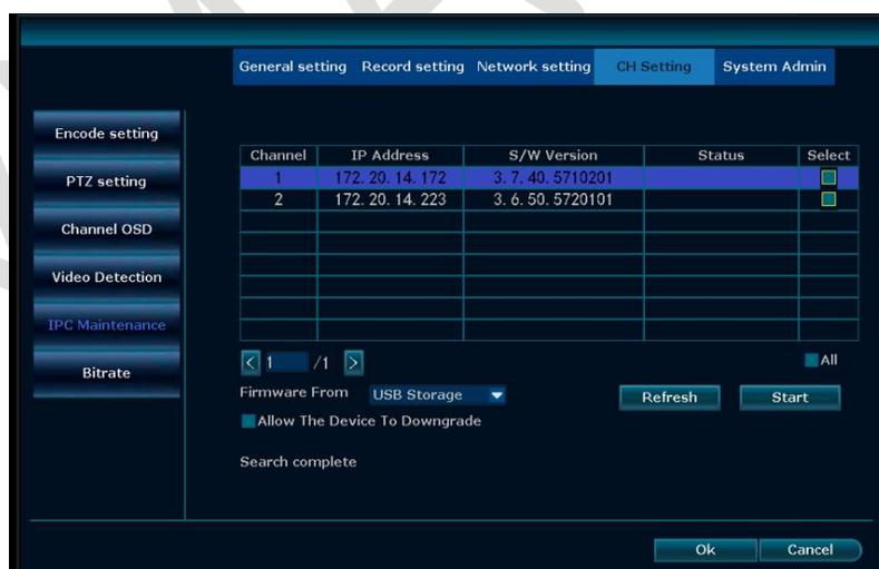
1. **Table:** Shows the IP and firmware version of all connected cameras.
