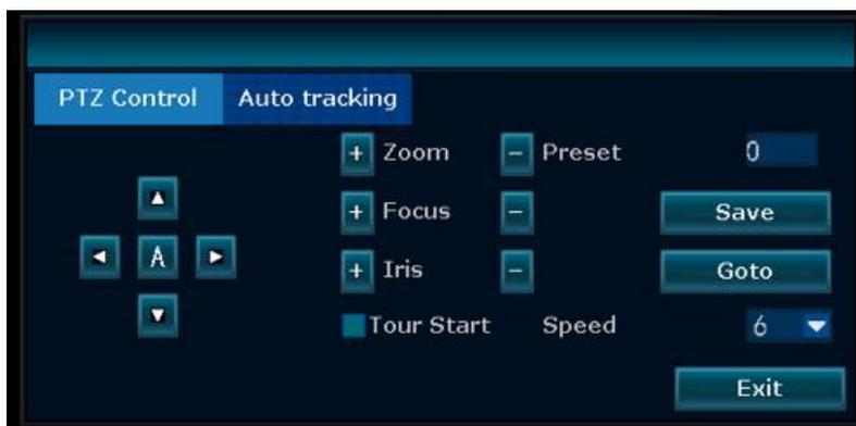
1. **Directional Arrows:** Click the directional arrows to manually control the movement of the camera. Click the button “A” in the middle to start an automatic scan, then tap on it again to stop it in the direction you prefer.
