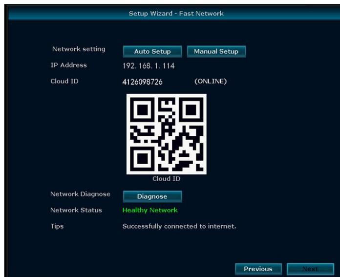
Fast Network will allow you to connect the NVR to Internet for remote access. You can either check DHCP to allow NVR obtain IP address from router automatically, or manually set an IP address for the NVR.
