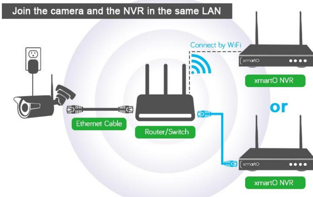
4. Add the camera to an NVR channel.
