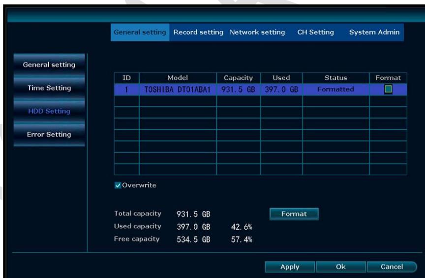
HDD Setting List of all the hard drives, including their characteristics, installed on the NVR.
