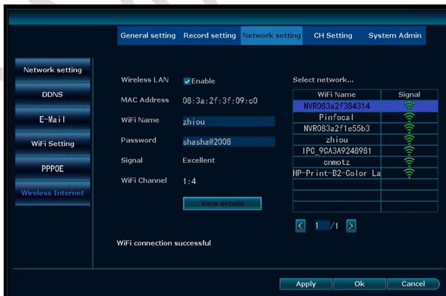
1. **Wireless LAN:** Check to enable and uncheck to disable it. Enable it, you can then set to connect NVR to your home network wirelessly.
