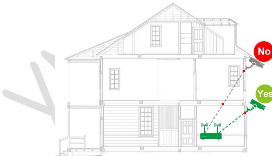
Always find possible open between NVR and camera, mount camera and place NVR's spot accordingly to allow signal to pass.
