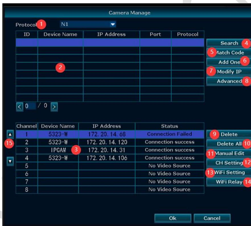
1. **Protocol:** Establishes the protocol used by the NVR when it is looking for cameras to pair with.
