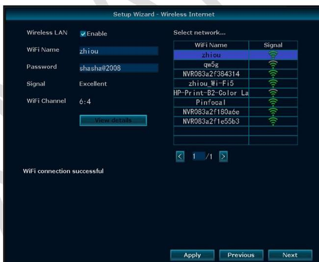
Wireless Internet will allow you to connect NVR to Internet wirelessly over WiFi. No need to hardwire NVR to router any more. Select the network WiFi name and enter the WiFi password, NVR will connect to your network wirelessly.
