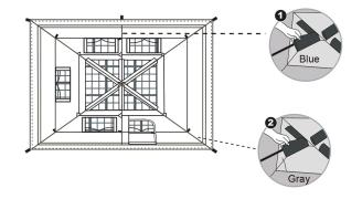
3. Distinguish between the middle and corner leg poles(Part E/F). Slide one end of a steel leg pole into the smooth end of elbow connector, then secure the other end onto the pin-rings at base of tent.
