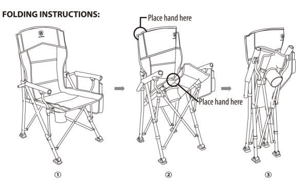
To Fold, place chair on even ground. Place one hand on the upper back side tube and the other hand on the lower seat side tube. Push the seat towards the back while leaning the chair slightly back on the rear feet and raise the front legs off the ground.
