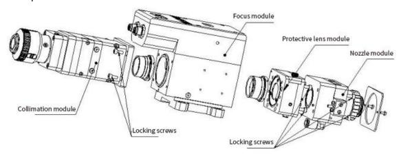
As shown below, use a lens removing tool to remove the focus lens mount.
