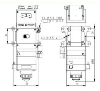
Fig 2.1 - mounting holes position
