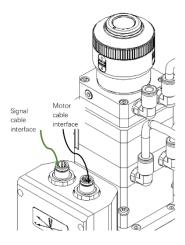
Fig 2.3 - cable interface of laser cutting head
