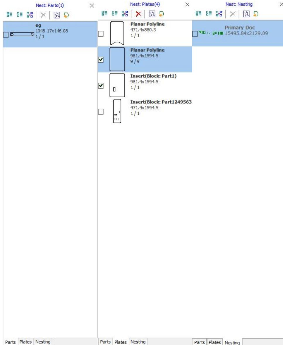
Parts library will list all parts, you can add new parts by right click at parts lib and select "load parts", or you can select parts at drawing board right click the part select "add to parts lib". The parts type limits is 50. Right click at side bar you can choose to import standard part, delete part or save un-nested parts.
