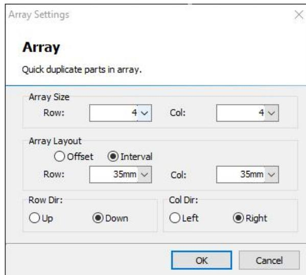
Set the rows, columns array layout and row direction of the array to duplicate the selected graphic:
