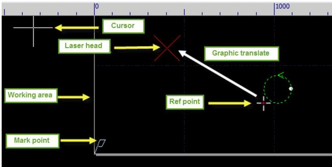
If the Red Cross does not match the real position of laser head, please check the mechanic origin and correct the origin by CNC-Return origin. If click "Preview" and graphic is partly or fully outside the white frame, it means machine will exceed the travel range.
