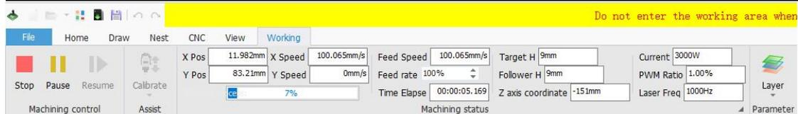
When in above status you cannot switch to other pages except File menu, for preventing graphics modified by mistake when machining. You can pause the machining to modify parameters, and it will take effect once machining resumed. If you modify without pausing the machining, the setting will take effect on the next one.
