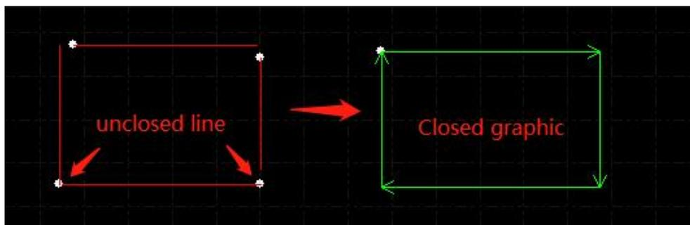
Please take notice that there might be excess line at geometry end, split and remove the excess line then combine the contour.
