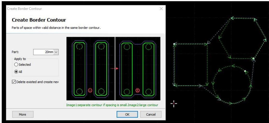
Parts distance: Parts of space within valid distance will be in the same border contour. The smaller the value is, the less parts will be contoured. It is recommended to set the distance longer than the actual one.
