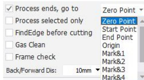
If " Process ends, go to" not selected, laser head will stand still at where finish the machining. If you want laser head return to a mark point, select "process ends, go to"+position you want.
