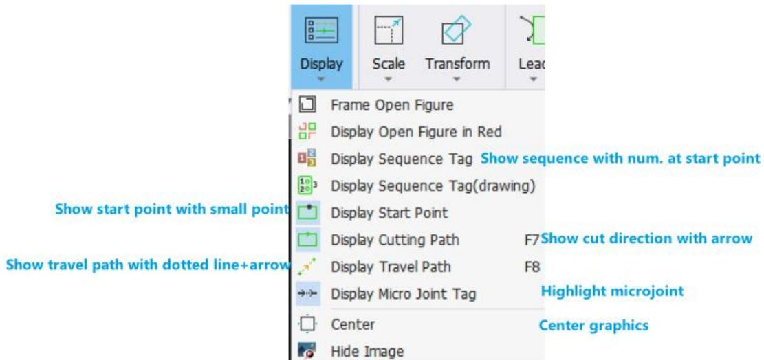
Click the button in the above picture, and the display will take effect immediately. You can see the change of the display in the drawing board. When the option button in dark gray, it is enabled, otherwise, it is not. For example, the on state
