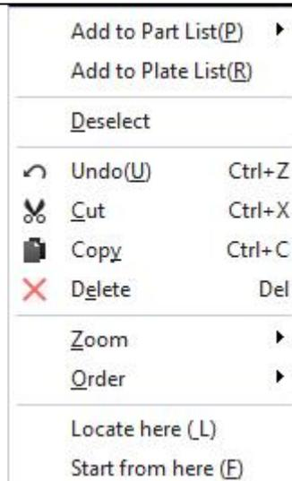
For safety concern, select "Start from here", program will prompt dialog box to ask users to confirm operation. Then laser head will locate to the specified position, and start machining. The path before specified position will not be machined.
