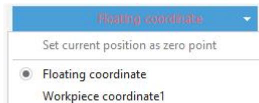
Click the button above the console panel you can select "Floating coordinate", "Workpiece coordinate" or "external coordinate".
