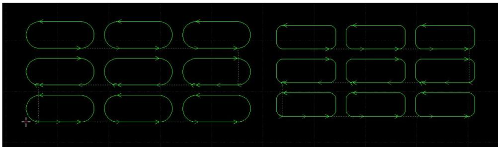
Select "Keep Micro Joint" when using Circular FlyCut and Obround FlyCut, the micro joints added before will not be cleared.
