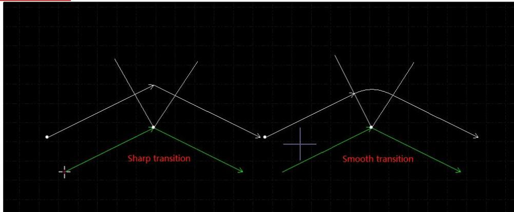
In the photo, the line of green is original graphic, white line is compensated path. It requires smoothing at corner. Usually round corner will smooth the machining path and assure the consistency of graphic and cutting result.
