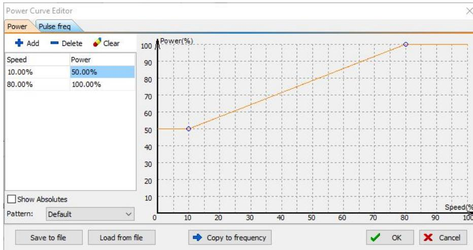
As shown in the photo above, horizontal axis is speed, vertical axis is power/frequency, unit is percentage. You can select the curve pattern and set the power level when machine reaches a specified speed. Or you can click "" copy the power curve to frequency curve. Notice: Only when "Power curve" is enabled, "Frequency curve" can take effect.
