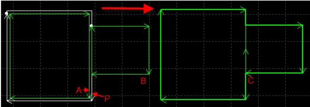
For example, in the above picture, graphic P is the compensation line of the graphic A, only graphic P can co-edge with graphic B because graphic A is not real cutting path.
