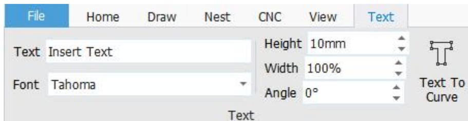
Please take notice that after turning text into curve, above functions will not be available. You would better finish all design and settings of the text before turning it into curve.
