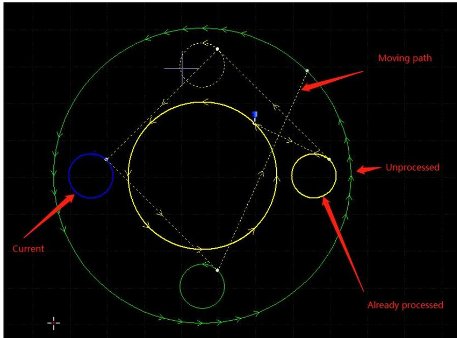
Sequence preview is completely interactive, making it easier to control the progress forward or backward, or zooming the graphics. You can view the move path to check the overall sequence by opening "View" drop down menu and select
