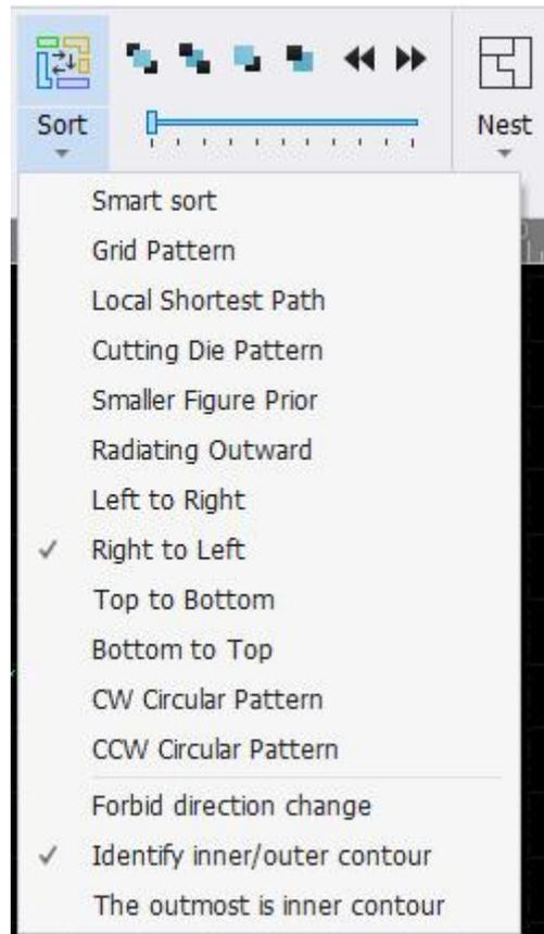
You can find details on group function in "Group". If no special requirement to the sorting result, "grid sort" is recommended.
