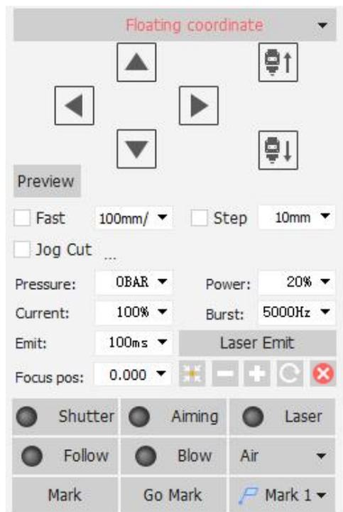
The button "●" will be in "●" once the function activated. Press "● Laser" will emit laser, release button will close laser; for other buttons, click the button activate the function, click again close the function. For example, click "● Blow" open the gas, click again close gas. For different laser model, there will be a delay
