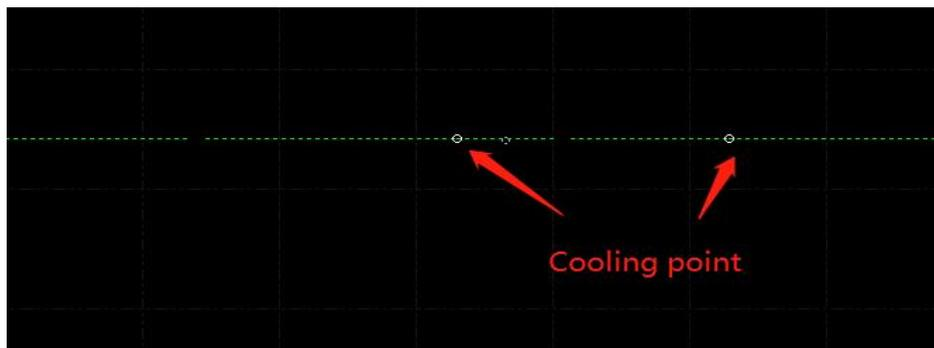
Like micro-joint, the cooling point can be clicked continuously to insert more than one. After you finish setting micro joint and compensation you can still add cooling point.
