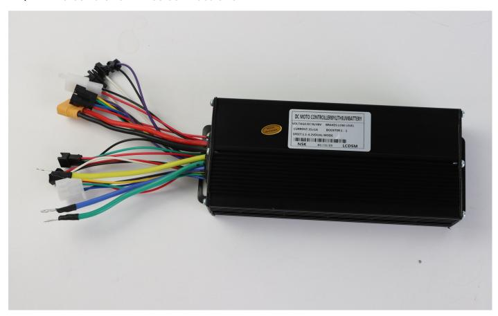
Motor cables connected to the Controller. **Note**: The thick three cables are the phase cables, should be tighten enough.
