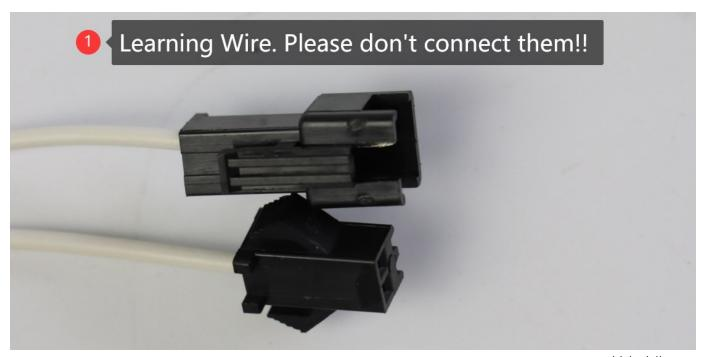
> This is a pair of brake levers or brake sensors connectors to the controller.
