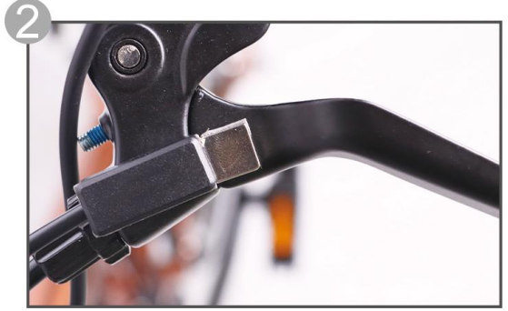
Install brake sensor
