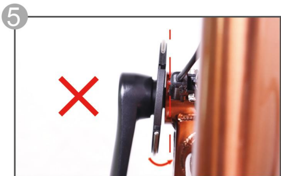
This is not correct because the signal is not continuous. The motor will not work well
