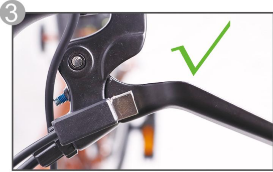
The magnet and sensor installed as close as possible
