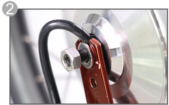
Place the tire and install the V brake (Note: The motor's cable is on the left side of bike) !
