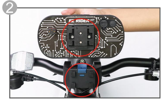
2 Snap the parts marked in the red circle together
