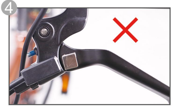
This is incorrect, the magnet and sensor are too far apart
