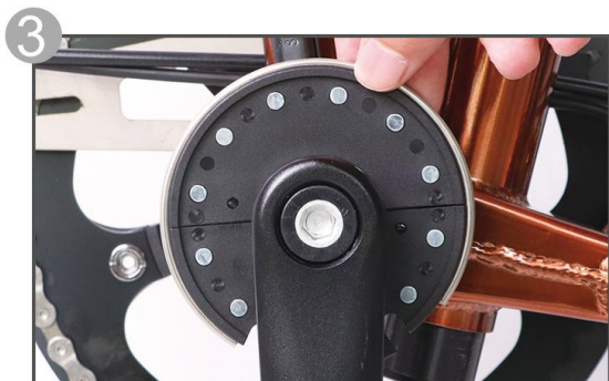
Install the retainer ring to fix the D12L PAS plate
