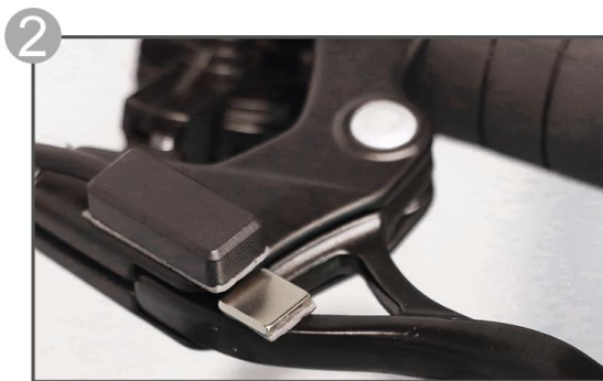
2 Install brake sensor
