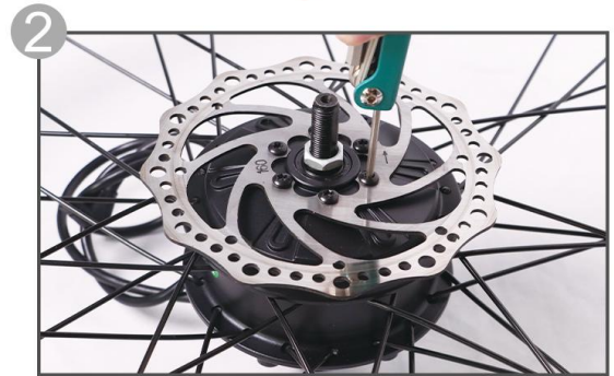
Install and tighten the disc screws
