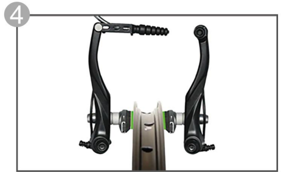
4 The correct position for the brake arms is where the rim is equidistant between both pads
