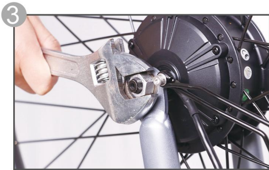
3 Tighten the screws, the motor wire spring must be inside the shaft
