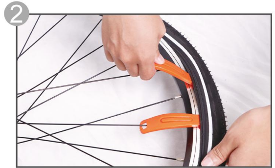
Remove and install tires
