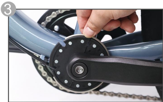
3 Install the retainer ring to fix the D12L PAS plate
