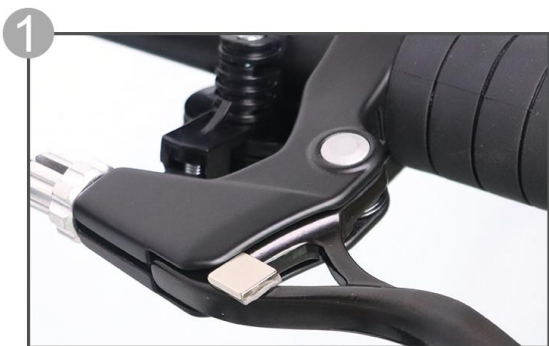
1 Install magnetic discs
