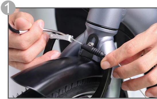
1 Release the V brake
