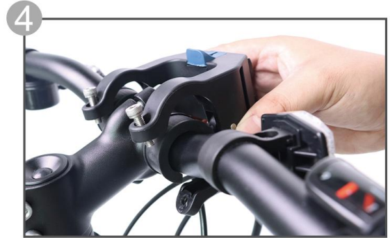
The bracket is installed on the handlebar
