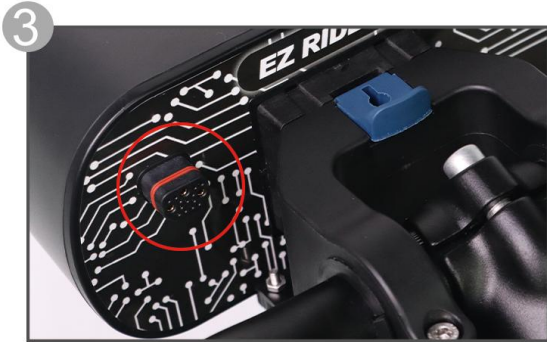
Controller battery wiring hole
