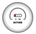
2. After turning off the vacuum, the battery indicator flashes in orange, then flashes slowly for 5s and goes out, indicating that the power is less than 25%, please charge it in time.
