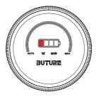
If a wrong adapter is being used, the battery indicator flashes red and goes out after 60s. The input voltage/current does not match, which will cause damage to the battery pack. Please replace the original adapter in time.
